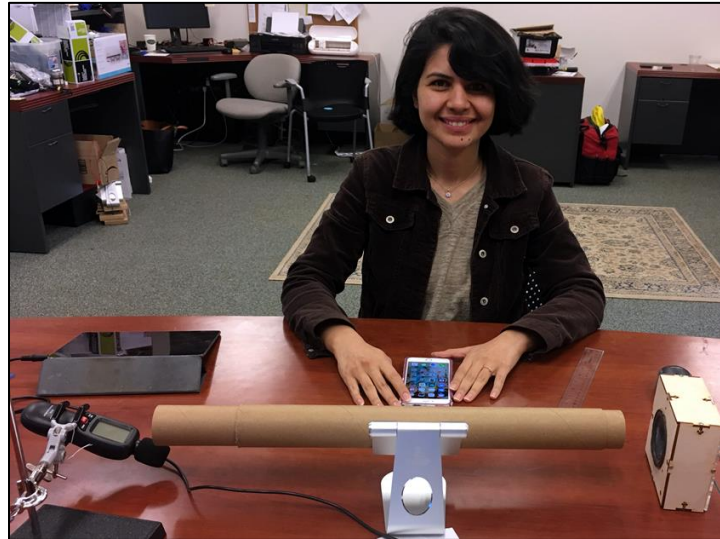
Figure 6. Measuring the amplitude of a sound wave traveling through a tube.
