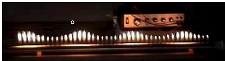
Figure 4. A Rubens tube can be used to visualize areas of high and low pressure.
