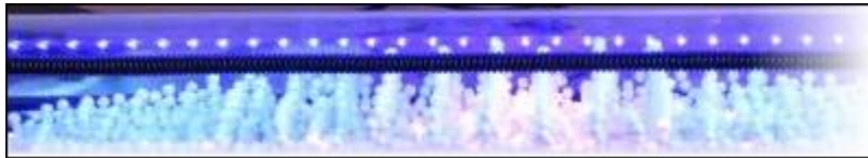
Figure 3. A sound wave traveling through Styrofoam suspended in a tube.
